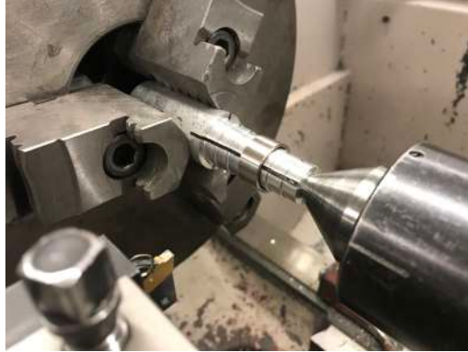
Ring chuck, being used to machine ring
